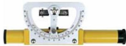
The Abney Level is an engineering instrument which can be used to determine height. It is moderately expensive and of medium size and weight.
